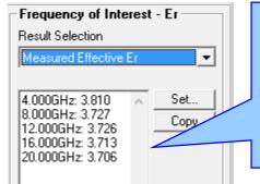
Using the same Frequency of Interest values of 4, 8, 12, 16 and 20GHz, the imported measurement data is examined and the effective dielectric constant values at those frequencies are displayed here
