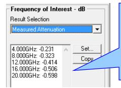
In this example the Frequency of Interest values have been set to 4, 8, 12, 16 and 20GHz. The measured attenuation (brown data series on the plot below) is examined and the dB loss values at those frequencies are displayed here
