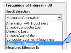
When importing insertion loss measurement data from the Polar Atlas it is often useful to know the exact measured attenuation dB values as specific frequencies. The new Result Selection options have been introduced to achieve this.
