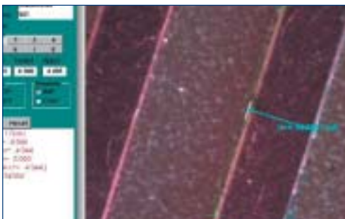
The Precision Line Gage system measures the top conductor line width and the line space at the same time.
