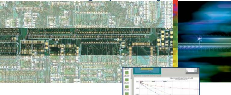
Design system for PCB layer stackup combined with PCB transmission line field solver.
