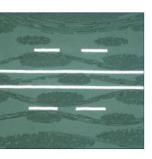
This photograph illustrates a polished microsection of a typical glass resin composite structure. This is FR4 but could equally be any woven glass reinforced composite. Glass has a dielectric constant of 6, the resin around 3. With high frequency base materials the resin Er can be even lower. On fine geometry boards with differential traces, local variations in the material Er need to be taken into account to obtain the most accurate prediction of impedance.
