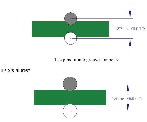
The pins fit into grooves on board.
