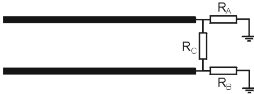
Fig 2a Typical Pi termination for a coupled line pair
