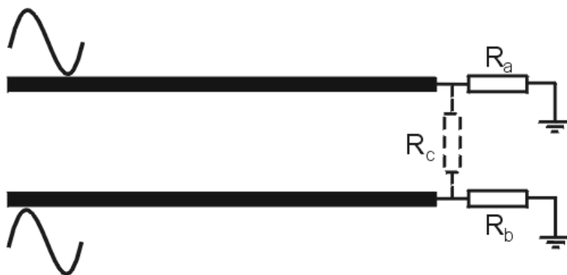
Fig 2b Equivalent termination (showing R c open circuit) in even mode
