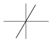
Suppose a large transient severely damages the protection diodes so that the circuit appears as a simple resistor; the signature is dramatically altered and very easy to see - the device is an obvious candidate for replacement
