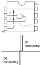
Damage to the I/O region of a digital device will be easily revealed using ASA. Consider the typical digital ic input protection circuit shown below
