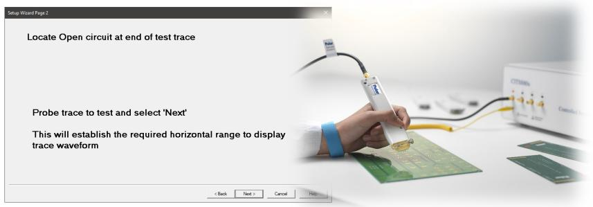
Ensure you have the ground pin of the probe aligned with the ground pad of the coupon before proceeding.
