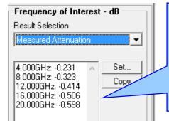
In this example the Frequency of Interest values have been set to 4, 8, 12, 16 and 20GHz. The measured attenuation (brown data series on the plot below) is examined and the dB loss values at those frequencies are displayed here
