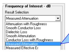
When importing insertion loss measurement data from the Polar Atlas it is often useful to know the exact measured attenuation dB values as specific frequencies. The new Result Selection options have been introduced to achieve this.
