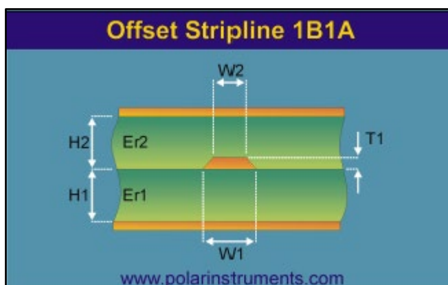
Offset stripline with one layer of dielectric above and below the trace
