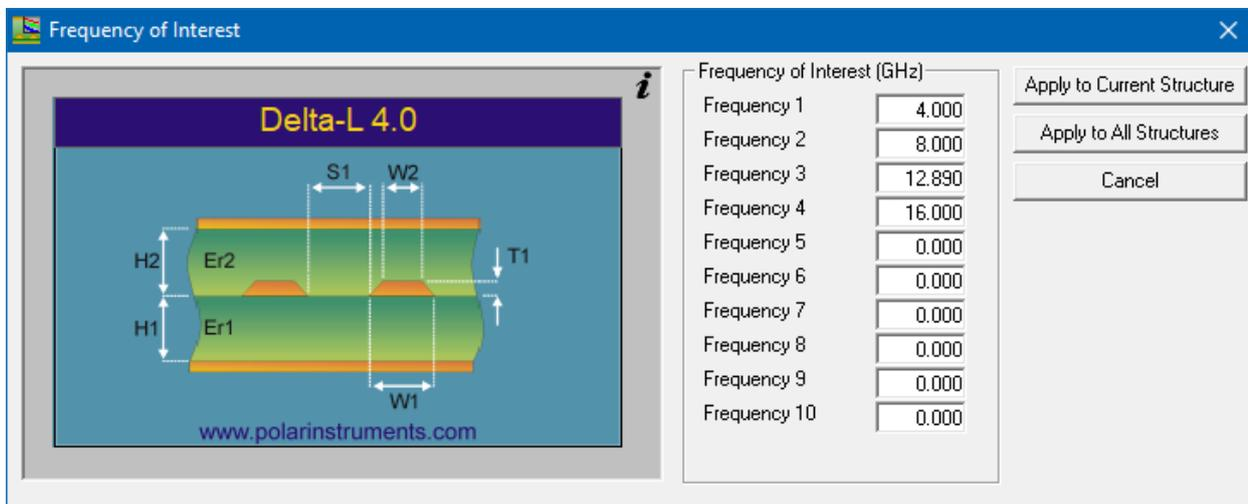
With all frequencies of interest defined, click on Apply to Current Structure (or Apply to All Structures to apply all frequencies of interest to all structures within the project.)
