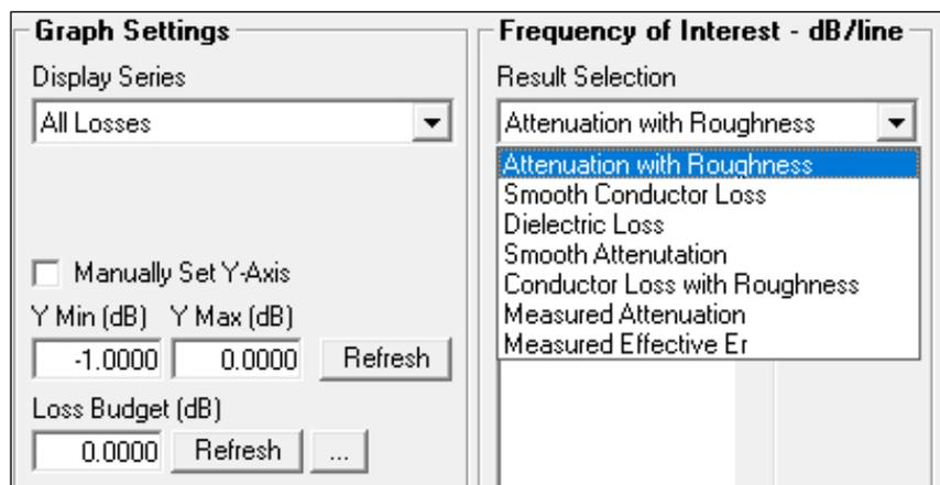
The readings in this example have been derived from measured data, so for this example it will be necessary to choose Measured Attenuation from the Result Selection dropdown in the Frequency of Interest pane.
