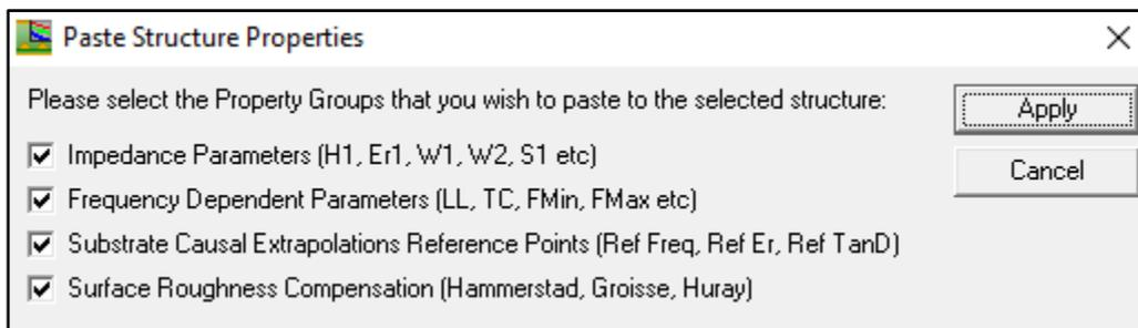
Choose which groups of properties are to be pasted into the field solver and click Apply. The impedance, lossless and frequency dependent properties are pasted into the field solver for processing. The units setting in Speedstack will replace the setting in Si9000e.
