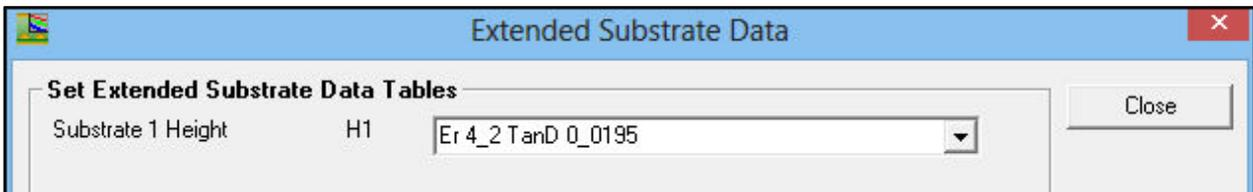
Close the dialog and Calculate – the Si9000 implements causal modelling using the Svensson-Djordjevic dielectric loss model.
