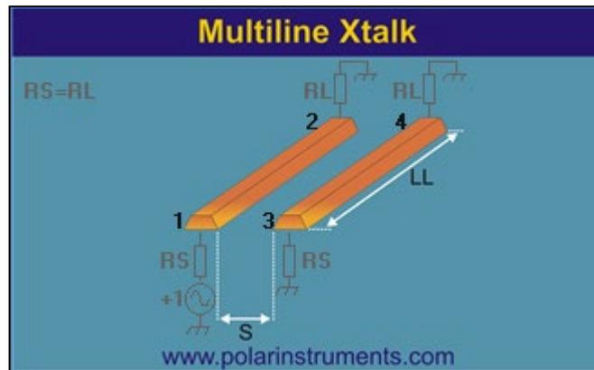
Choose the aggressor and victim lines and voltages. Supply the parameters, line length, separation, etc. for the model:
