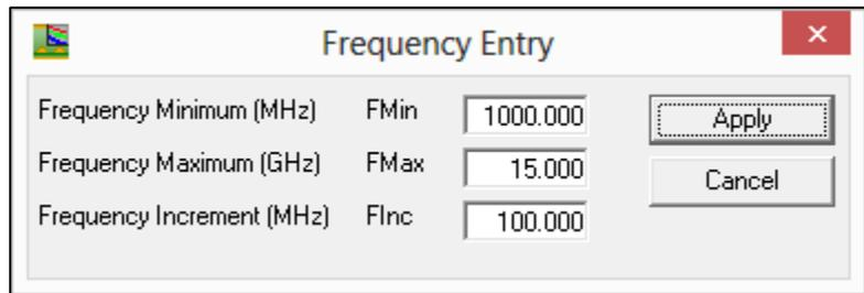
It will be necessary to recalculate to reflect the new settings. Click Apply and then click the Calculate button
