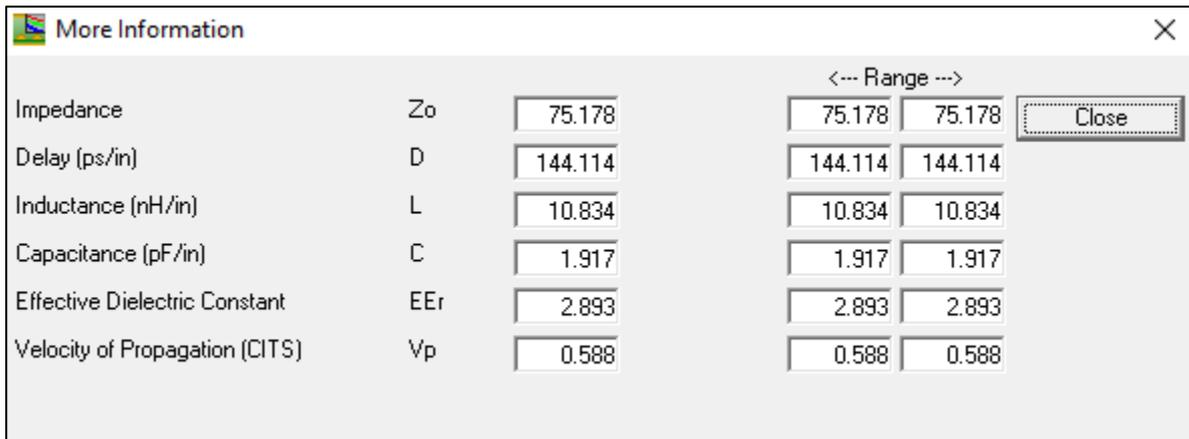
The More Information dialog displays the results of impedance, propagation delay, inductance and capacitance along with effective Er and velocity of propagation (useful for Test Editor | Vp entry within the Polar CITS test editor) in the selected units. Press **Close** to exit.
