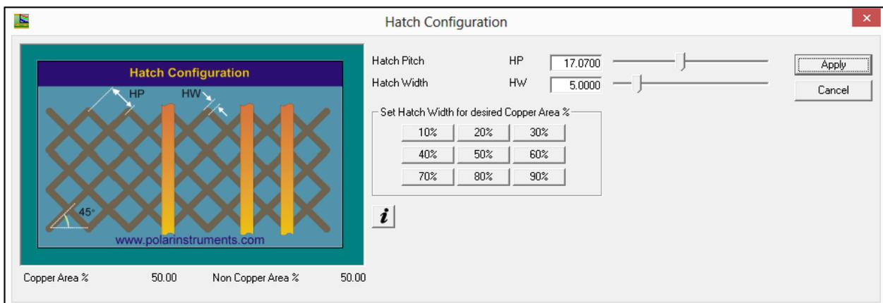
The XFE option, applicable to the lossless mode of the Quick Solver allows for configuration of hatch pitch (HP) and
