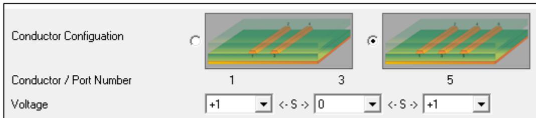
The aggressor and victim lines and associated ports for the selected conductor configuration are reflected in the accompanying graphics as shown in the dialogs below.
