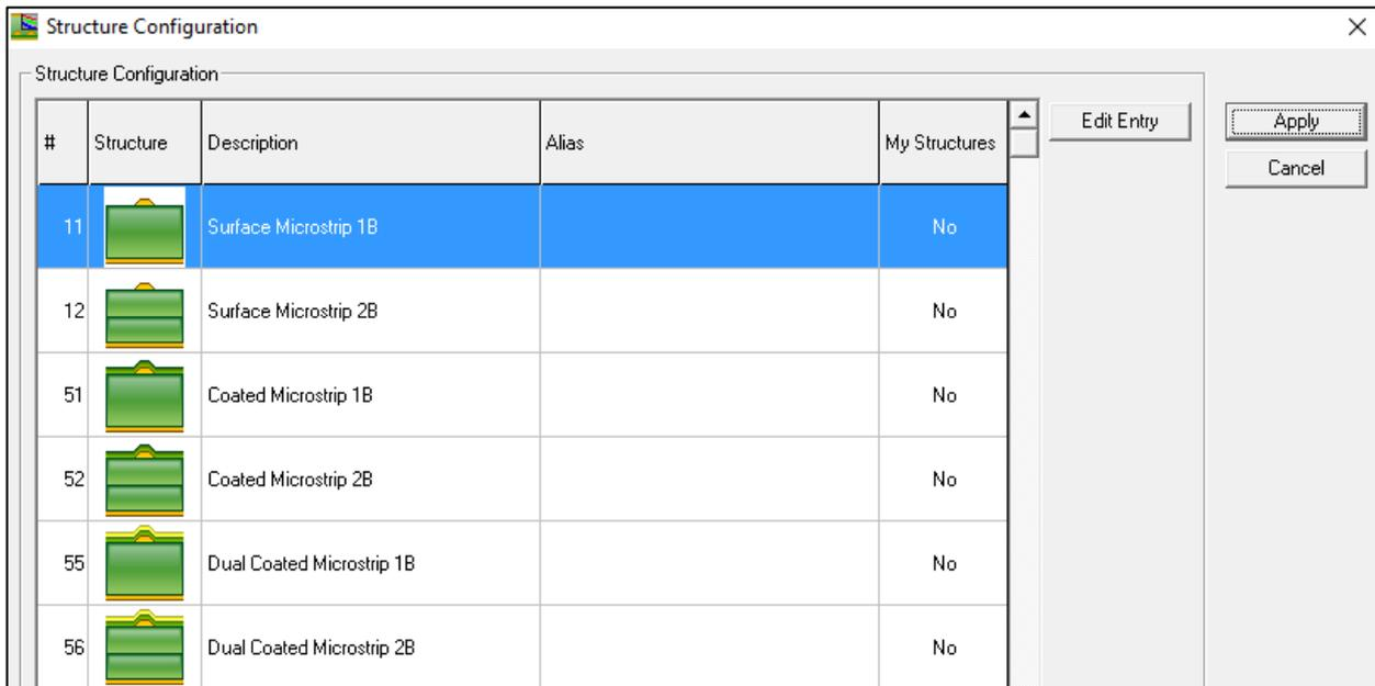
Add the descriptive text to provide a label for the structure in the Alias field:
