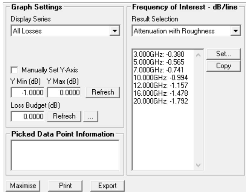
Frequency of interest settings can be applied to the current structure or, for example, all the structures within a project.
