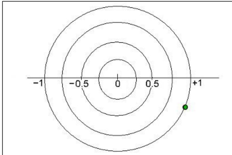
Where this dot is plotted would depend on the phase shift through the transmission line. If the frequency were increased, and other  $S_{21}$  frequency readings obtained, the magnitude of  $S_{21}$  would still be 1 but the phase shift would change.
