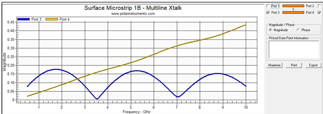
Change the, line length, separation, frequency, etc. to examine the effect of changing parameters on near and far end crosstalk.
