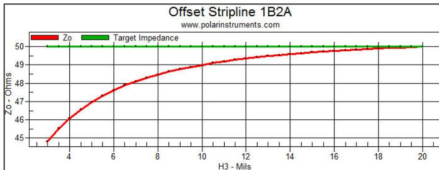
The chart displays the impedance varying between 45 and 50 ohms as H3, the distance to the interstitial copper leaf, varies between 3 mils and 20 mils.
