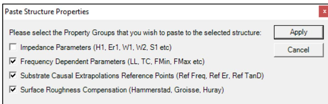
Select the properties to be pasted – in this case, the impedance parameters are unchecked as the source structure’s 100 ohm differential impedance does not apply.
