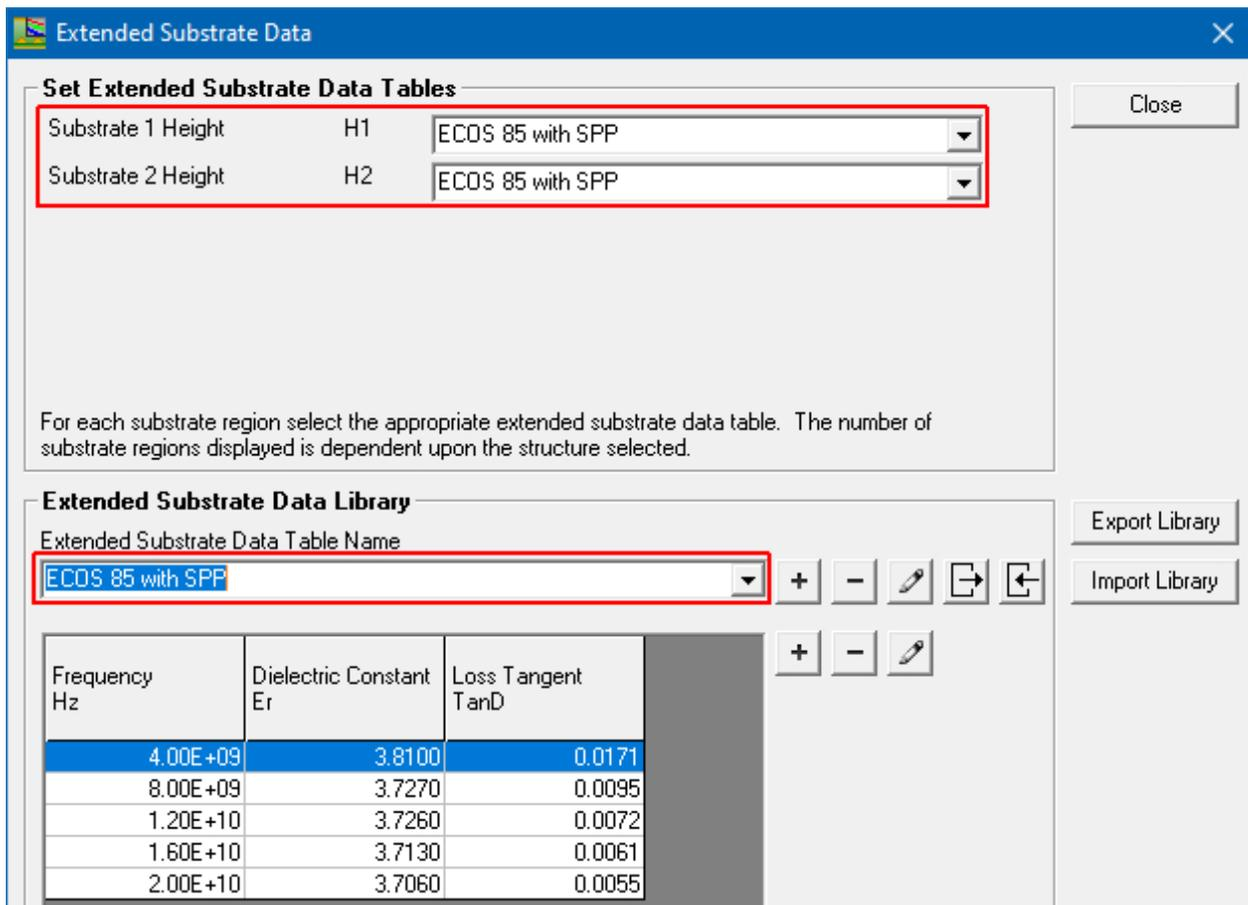
The table data may be used as described in *Using Extended Substrate Tables*. Multiple frequency goal seeking uses the data contained within the specified table.
