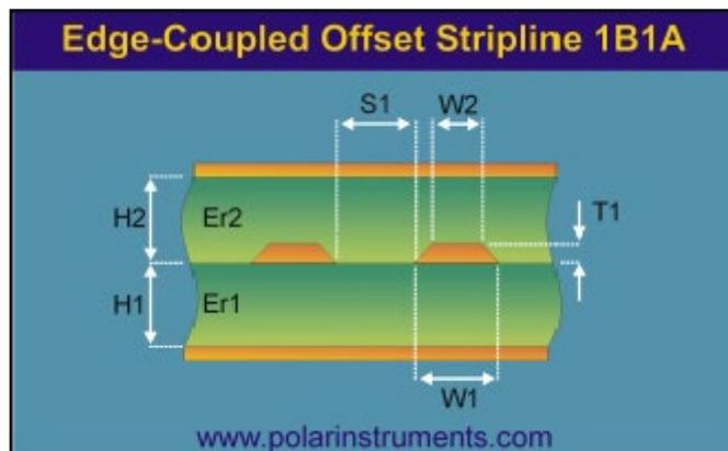
Enter the parameters below and goal seek on trace width for a differential impedance of 75 Ohms.
