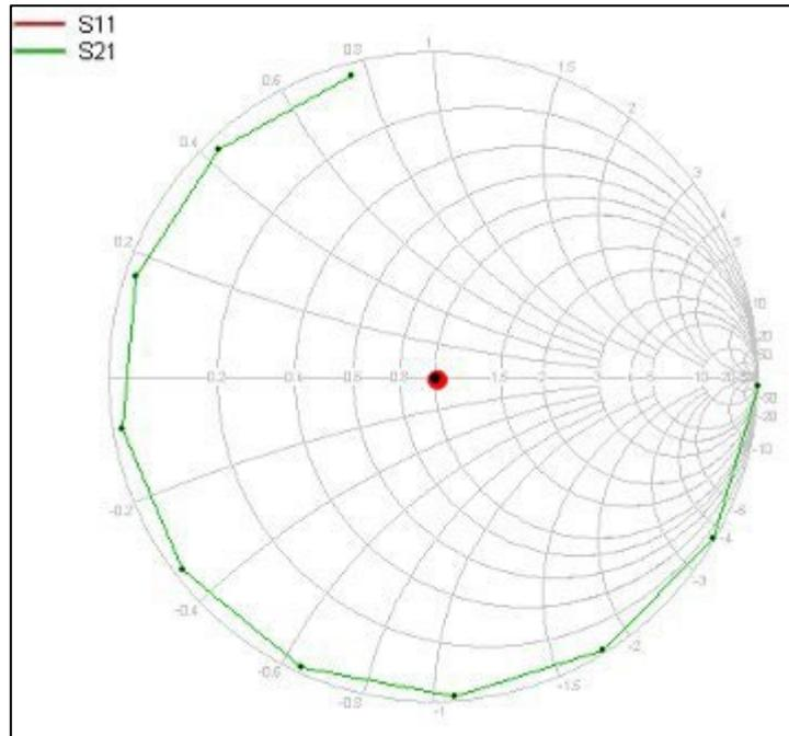
The previous graphs plotted an ideal network with no loss. This plot shows this transmission line with a small amount of loss, as the 15GHz point is no longer sitting on the unity outer circle. If the loss increases with frequency the reflection coefficient becomes smaller and the plotted line spirals inwards.
