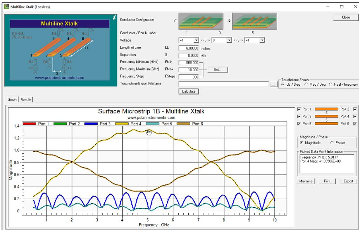
The coupling is modeled against frequency and line length and allows a designer to plan for enough trace separation between individual signal lines or between differential pairs for crosstalk to be within safe limits. Both *near* and *far-end* crosstalk are modeled for stripline and microstrip cases.
