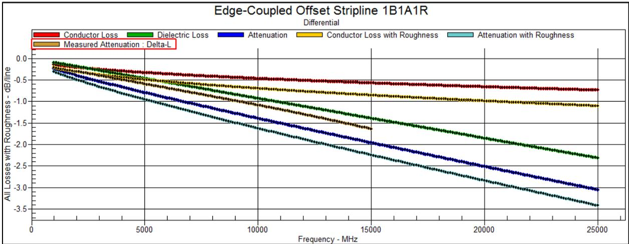
Comparing the Attenuation with Roughness curve with the Measured Attenuation indicates the degree of correlation.
