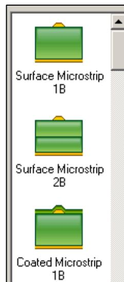
Use the Structure Bar to select a controlled impedance structure from the list of structures displayed. The range of structures displayed is controlled by the associated button on the Toolbar.
