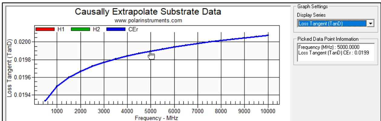
Click a data point on the graph to display the value at the frequency of interest in the Picked Data Point box. Results may be displayed in graphical or tabular format.
