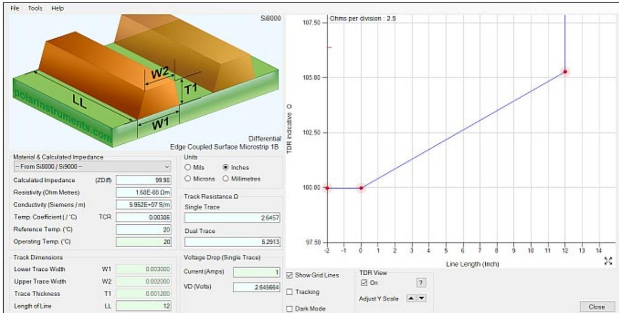
Example 2 – 3 mil line width 100 Ohm differential pair with 5 Ohms DC resistance
