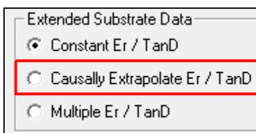
For this example, choose the Causally Extrapolate Er / TanD option from the Extended Substrate Data option group to apply Svensson-Djordjevic modelling to each dielectric layer in the current controlled impedance structure.
