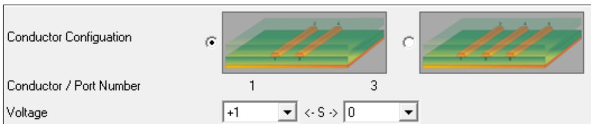
The Crosstalk graphic displays the two lines and four ports associated with the model.
