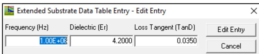
To use the new table, select the table from the dropdown list in the Set Extended Substrate Data Tables section of the dialog.
