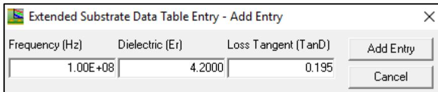
Each band is added to the table in ascending order of frequency. In this example the dielectric constant, Er decreases with frequency, but loss tangent, TanD remains constant.
