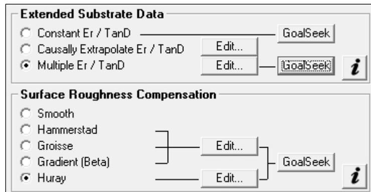
The Loss Tangent Multiple Frequency Goal Seek dialog is displayed. The dialog allows for up to five Loss Tangent values to be calculated in a single process.
