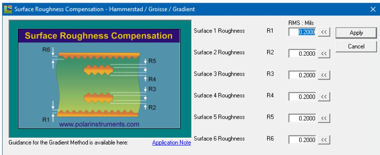
Values for surface roughness (obtainable in consultation with the board manufacturer) are specified in the currently chosen units. Typical values for RMS roughness could be  $0.8\ \mu\text{m}$  (0.03mils) for stripline,  $1.6\ \mu\text{m}$  (0.06mils) for surface microstrip. The Si9000e assumes losses on all sides of a copper trace.
