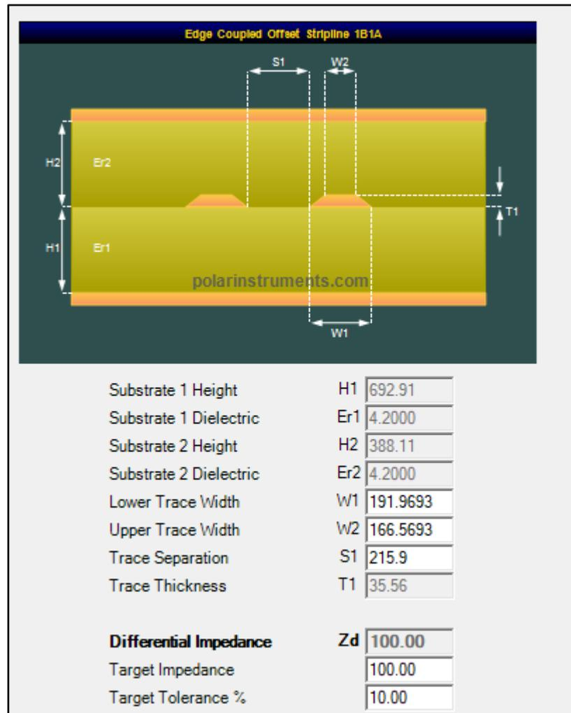
Rebuild and recalculate to refresh the stack. It may also be necessary to round some dimensions (e.g. dielectric heights) to the nearest practical values and recalculate the impedance
