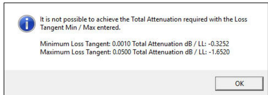
The minimum and maximum Loss Tangent values as specified in the Setup Goal Seek Parameters are displayed along with the calculated Total Attenuation.
