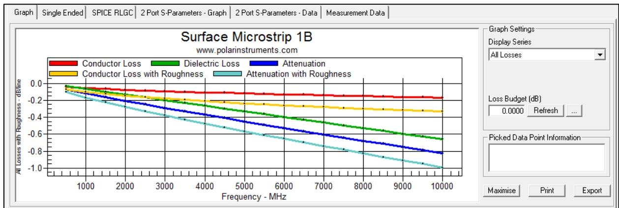
Options and parameter settings for the presentation of frequency dependent data include: linear or logarithmic scales, units (inches/meters) for line length,  $E_r$ /TanD options, user-editable surface compensation methods, measurement data options, s-parameter configuration.
