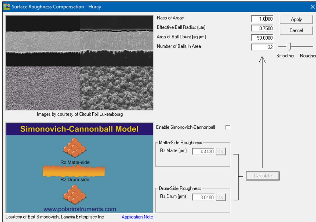
Supply the values in the associated fields and click Apply. If the Huray values are not available, click Enable Simonovich-Cannonball and supply the Rz values for matte and drum side roughness and click Calculate to populate the Huray fields, then click Apply. Click Calculate to refresh the graph.
