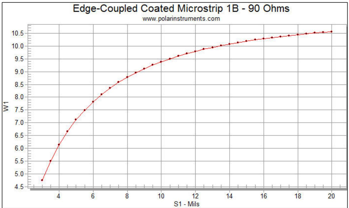
A subset of the sensitivity analysis results as trace width and separation vary is shown below.
