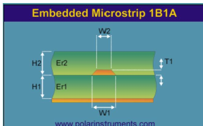
Embedded microstrip with two dielectric layers, one below and one above the trace
