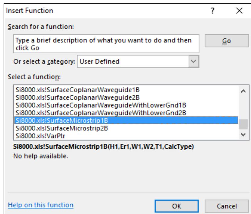
If necessary, scroll to the controlled impedance structure functions; click the function associated with the surface microstrip structure (Si8000.xls!SurfaceMicrostrip1B in this example) and click OK: the Function Arguments dialog is displayed.
