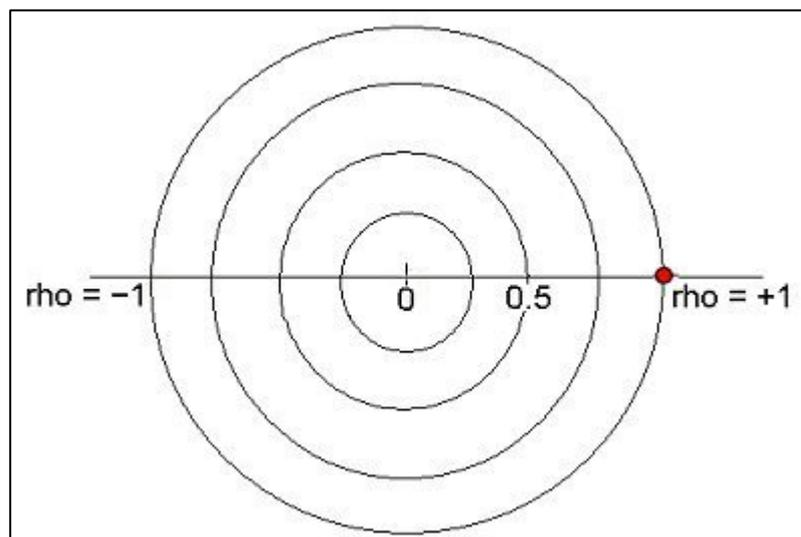
Similarly, a point plotted at right-hand edge shows 100% +ve reflection, i.e. unity reflection with no phase change, implying a transmission line terminated with an open circuit.
