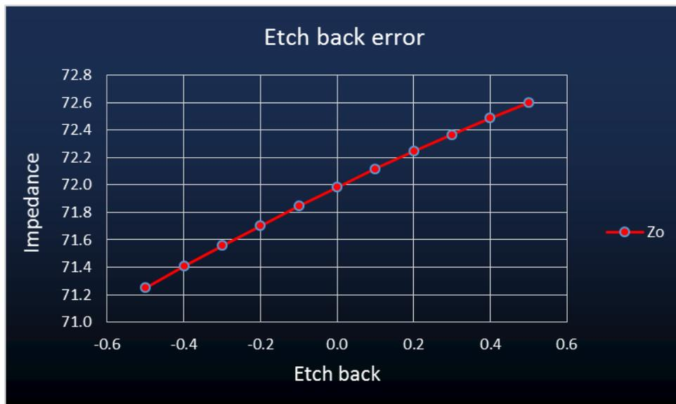
Change the etch back factor cell value in cell C53 and recalculate to observe the change in impedance of a different trace side slope.
