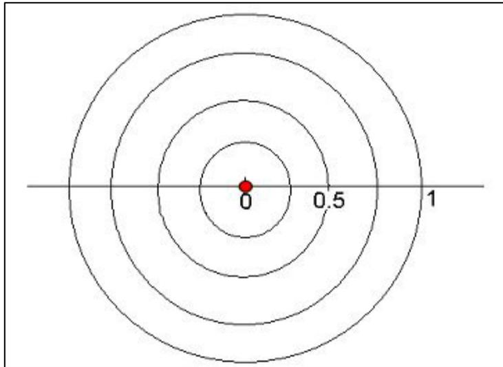
A point plotted at the origin shows no reflection, i.e. a transmission line perfectly terminated.
