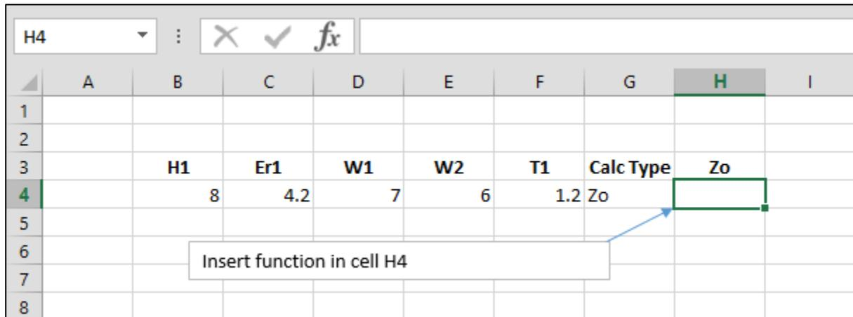
Construct the model as show above and click the **Insert Function** button on the formula bar.
