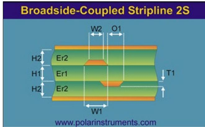
Note the *six surfaces* for the broadside-coupled stripline structure, and their associated values for roughness.
