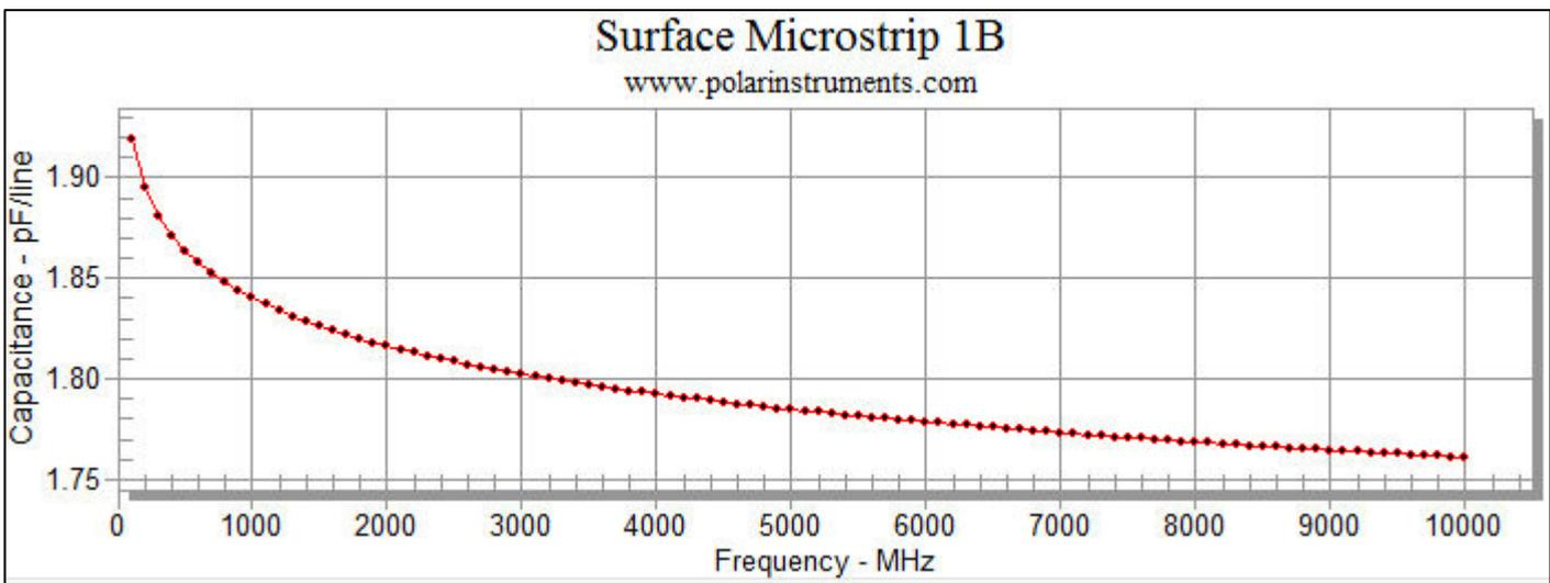
Note that the Si9000e applies frequency dependent permittivity modelling even though Er and TanD are specified with single values (i.e. as constants.)
