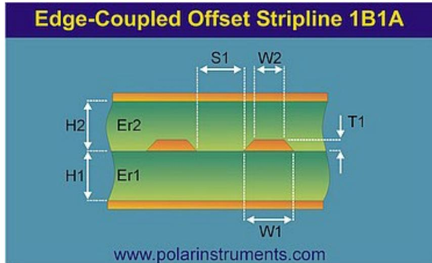
On the Lossless Calculation tab, supply the structure parameters and calculate the impedance.
