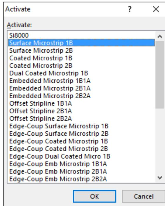
Select the structure from the list. Scroll through the list to display all supplied structures.
