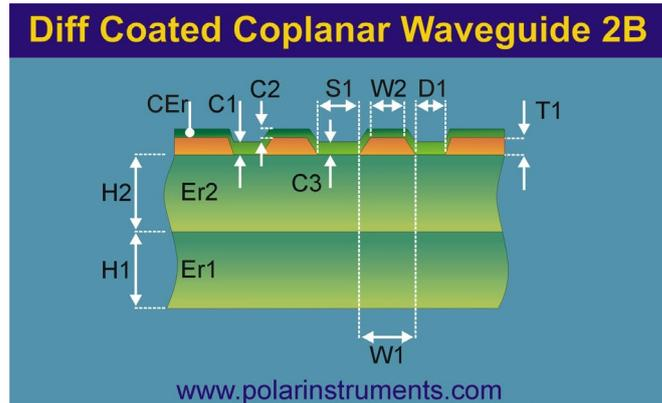
The diagram above shows a differential coated coplanar waveguide fabricated using two dielectric layers.
