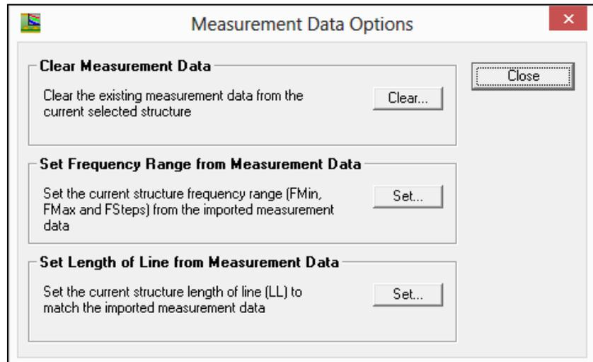
The new settings will be applied after the dialog box is closed. It will be necessary to click Calculate to update results.
