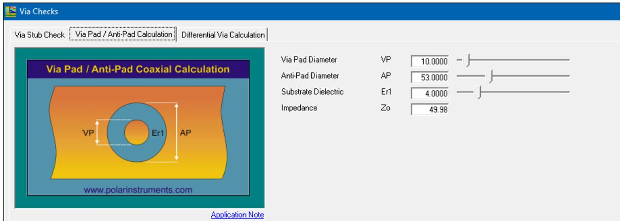
The anti-pad is the void area (shown as the blue annular ring in the diagram below) between the pad and the copper of the plane. It should be designed so that it maintains the impedance of a transmission line as it passes through the plane.
