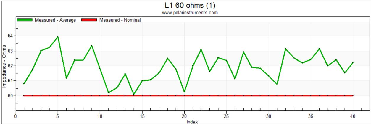
The chart above displays the logged measured data for each board along with the nominal impedance value.
