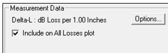
Measurement data may be optionally included or excluded from the All losses plot via the associated check box.
