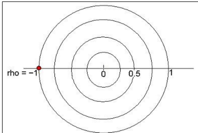
Commonly, a point plotted at the left-hand edge shows 100% –ve reflection, i.e. unity reflection with 180 degrees phase change, implying a transmission line terminated with a short circuit.
