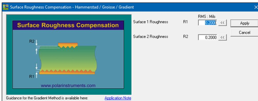
Roughness values may be set for each surface in the structure – *two surfaces* in the surface microstrip structure above.
