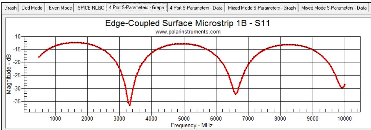
Choose from the Graph Settings Display Series drop-down list to choose results, including those for loss, impedance, inductance, resistance, capacitance, conductance, skin depth and attenuation and effective Er.
