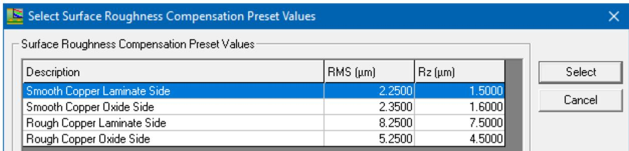
*Note that the roughness values in the table are shown in microns regardless of the parameter entry units chosen.*
