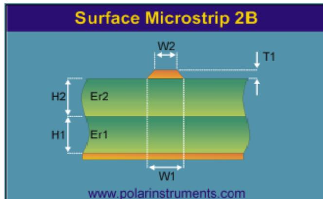
Surface microstrip with two dielectric layers below the trace
