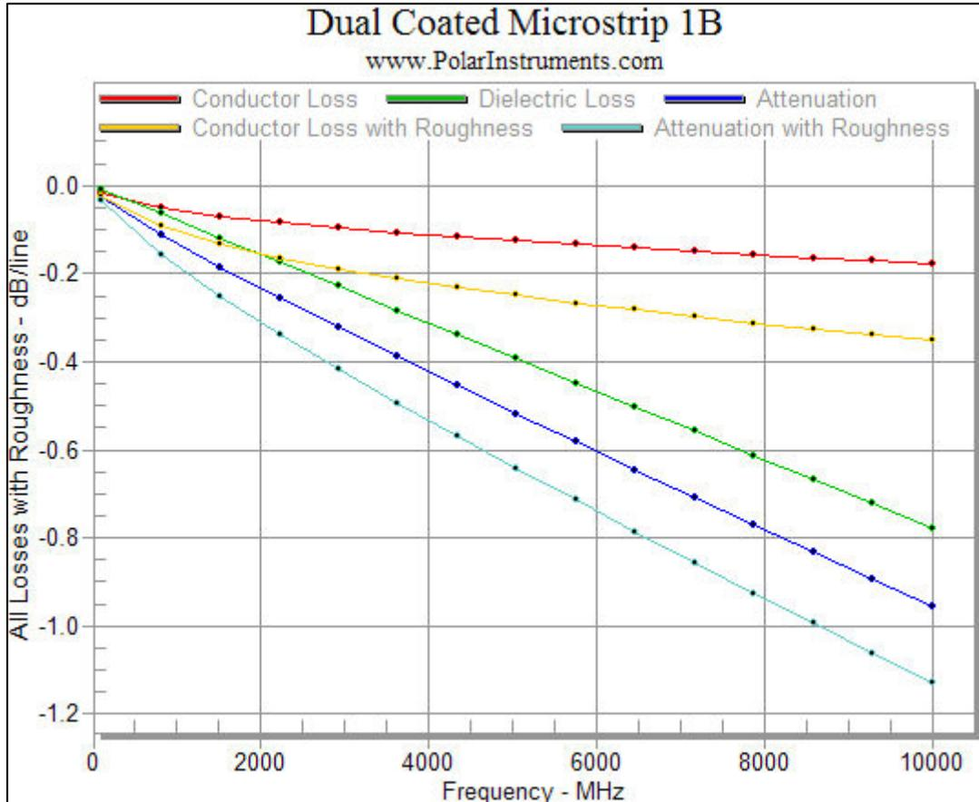
The Si9000e graph above charts all losses, the dielectric loss and the significant increase in the overall loss due to surface roughness, allowing the materials supplier to isolate the contributions of the different loss mechanisms.
