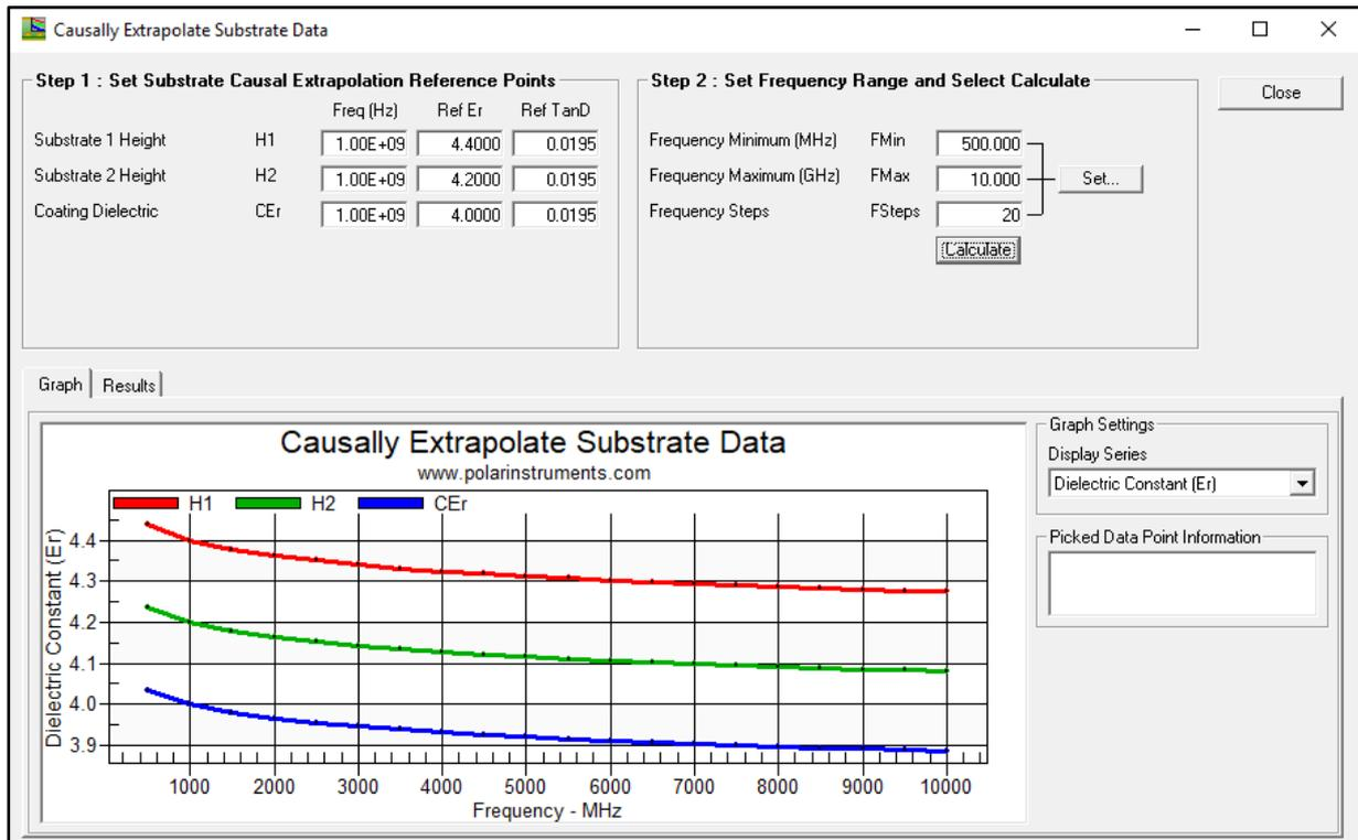
Each substrate in the controlled impedance structure may be assigned causal extrapolation reference points.
