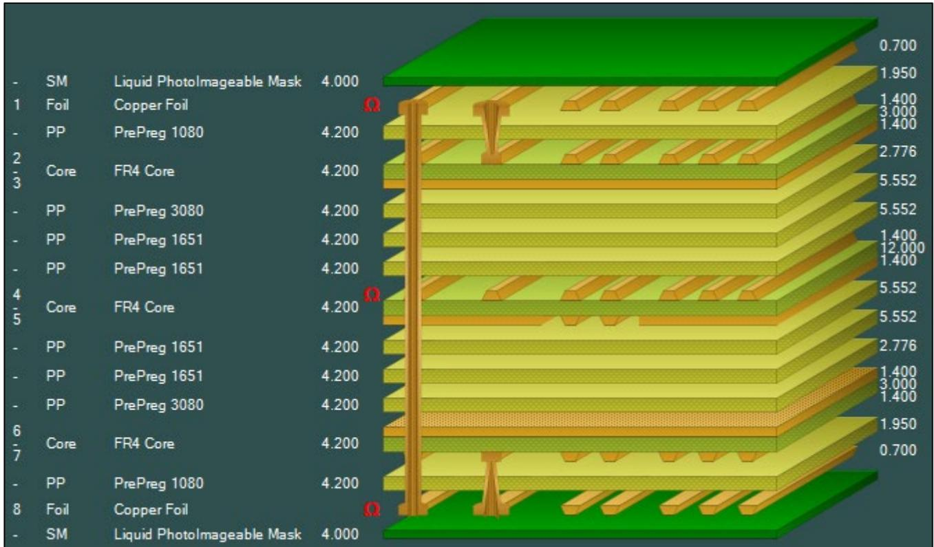
Click Speedstack's Controlled Impedance tab to display the structures.
