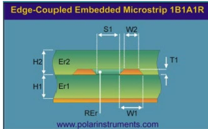
Edge-coupled embedded microstrip with resin-rich region between traces
