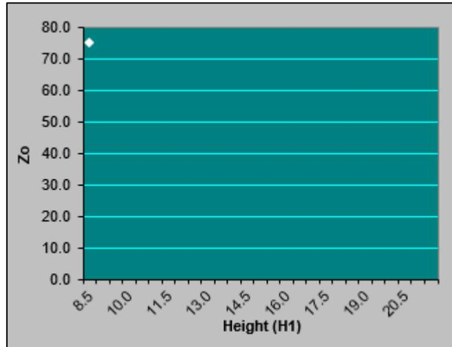
To chart the change in  $Z_0$  (or  $D$ ,  $L$ ,  $C$  or  $EER$ ) as the height,  $H1$ , changes over a range of values, use the Excel Fill Handle to copy the function formula down into the associated cells.
