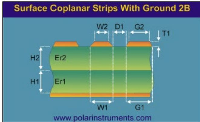
The diagram above shows a differential surface coplanar structure with strips and a lower ground plane fabricated using two dielectric layers
