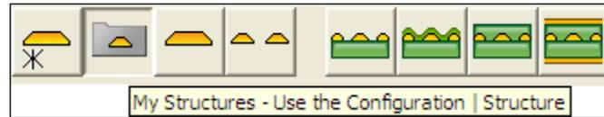
Choose the Configuration | Structures command to display the complete list of structures – select the structure to be edited and click Edit:
