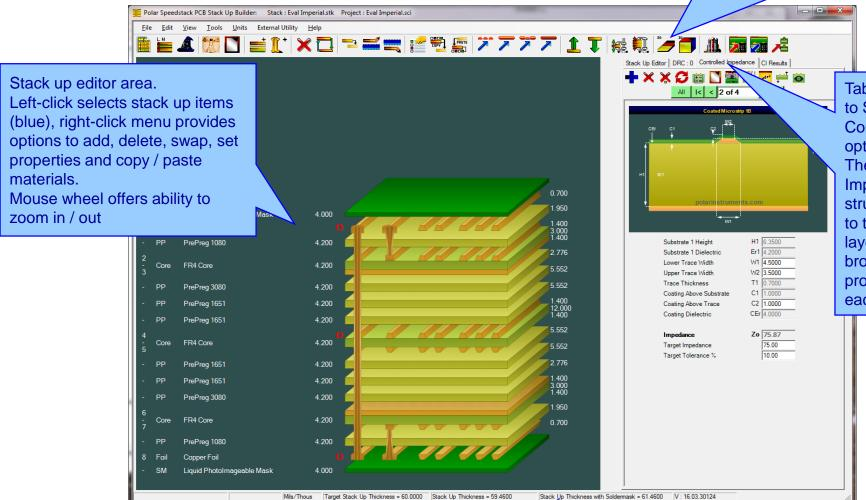
Tabs provide access to Stack Up, DRC and Controlled Impedance options.
