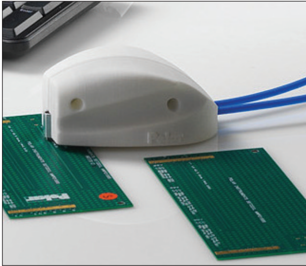
Ergonomic ESD safe GGB probe body
