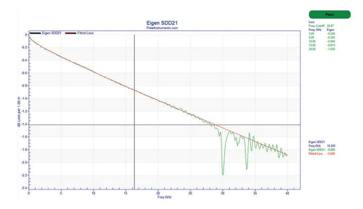
Stackup design environment Atlas Si is a precision insertion loss measurement package designed specifically for PCB fabricators and OEMs. It provides accurate, repeatable measurements of frequency based transmission line losses, allowing fabricators to meet stringent targets that maintain signal integrity within the limits of the latest high-speed chipsets.
