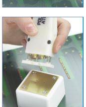
Atlas uses powerful mathematical processing techniques to allow nonskilled operatives to measure differential frequency-dependent losses from a test coupon quickly and easily. The system is easy to set up, easy to use and delivers fast results without the need for extensive operator training. A single insertion loss test can be performed in a couple of seconds, compared to minutes or hours using traditional techniques.
