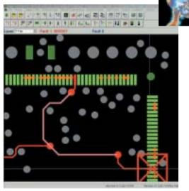
Easy for technicians to trace a faulty net as it disappears and re emerges from inner layers
