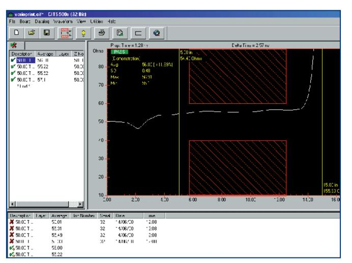
Test results are clear – the CITS100s automatically processes the data to produce a simple display of impedance versus distance, and reports a PASS or FAIL for each test.
