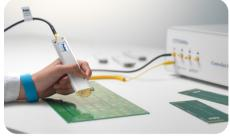
Handheld probes for on board or coupon-based controlled impedance test
