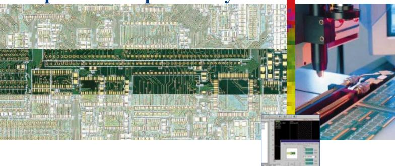
Automated impedance measurement for volume coupon testing with excellent R&R
