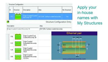
Simplifies transmission line modeling Over 100 transmission line structures Boundary element method (BEM) field solver Analyses single and multiple dielectric builds Includes solder-mask effects
