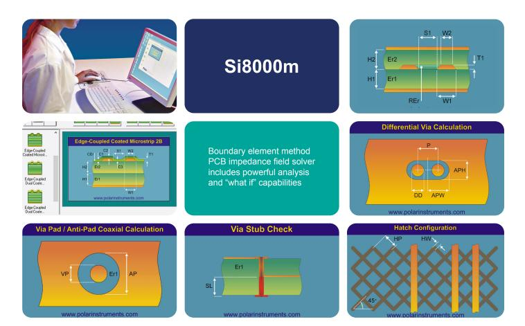
Accurate BEM impedance field solver Use with single and multiple dielectrics Predict manufacturing tolerance Sensitivity Analysis increases yields Model differential, common, odd mode and even mode impedance Goal seek on single or multiple parameters
