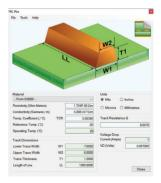
An optional track resistance calculator takes the geometric trace data from the Si9000e to quickly and easily calculate both track resistance and voltage drop for a given track length.
