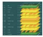
View stackup in 2d or 3d format. Layer and material annotation is clear and easy to read, each layer may be selected and queried to display the associated material type and properties, including the associated gerber file. Visible drill information ensures that designers instantly know which layers support blind and buried vias.
