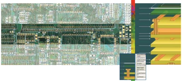
Design system for PCB layer stackup calculation and documentation
