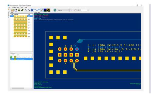
CGen is not only a stand alone coupon generator, but comes into its own when used alongside Speedstack PCB. CGen can directly import impedance controlled stackups and create the appropriate test coupon gerber files for your CAM department. By selecting coupons with Polar preferred footprints you minimise your need to invest in bespoke test probes for impedance test.
