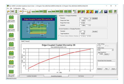
The Si8000m controlled impedance design system offers advanced field solving methods to model most track designs and is the natural partner of the Polar CITS controlled impedance test system. Si8000m allows fabricators and designers to explore transmission line design space before committing to build and document the full stackup with Speedstack. To assist the designer or fabricator new to impedance control, Polar's website is packed with informative application notes.
