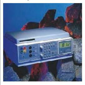
You then use a roving probe to touch any connection on the stimulated plane and follow the arrows on the front of the 950. Three or four movements of the probe are usually sufficient to bring you to the region of the short.
