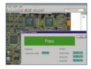
The FT100 uses impedance comparison techniques to help you faultfind complex pcbs.
