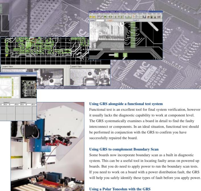
Once you have identified the failing net with the GRS, the fault may be quite obvious to you. However this is not always the case and to look more closely at a leaky or short circuited net, a Toneohm 950 (optional) is an excellent complement. The Toneohm is equipped with a variety of techniques for determining the physical location of shorts or components causing excess load. These techniques are covered in more detail in the Toneohm 950 literature.
