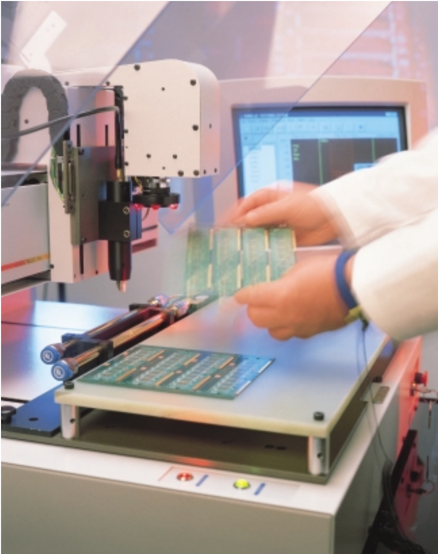
Figure 4. Automated Impedance Test.
