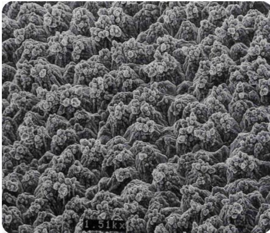
Figure 2 SEM photograph of electrodeposited copper nodules on a matte surface resembling “snowballs” on top of heat treated base foil. Photo credit Oak-Mitsui.
